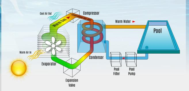
The hot vapour enters the titanium heat exchanger condenser where it transfers its heat to the water. As the vapour cools, it condenses back into a liquid, and releases its latent heat to the water passing over the heat exchanger condenser unit. Exiting the condenser, the cold liquid refrigerant is under high pressure. The refrigerant passes through an expansion valve that reduces the pressure and allows the refrigerant to re-enter the evaporator to begin a new cycle.
